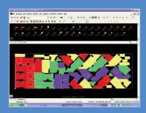
Part data is entered directly into the CAD system and is ready for editing and/or nesting
