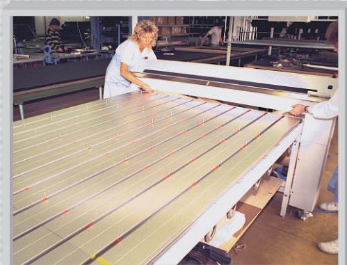
separate needles can be switched on and off
