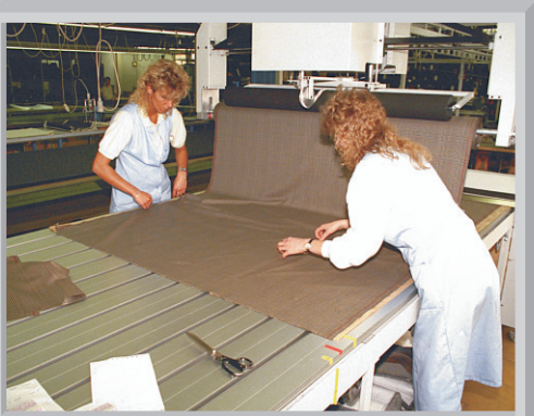
spreading the fabric and matching it in one step
