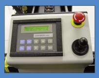
The easy-to-use keypad controls many machine functions at the cutter.
